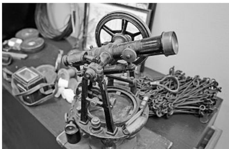
Supervisor Pat McMichael displays surveyors tools from precomputer days in his office — a transit (left) for measuring angles and a cloth measuring tape (right).
